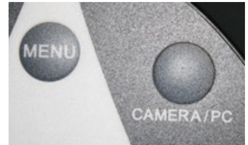
The Camera/PC button is used to toggle between the camera and a laptop or PC computer display.
