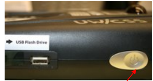
The Power button for the camera.
